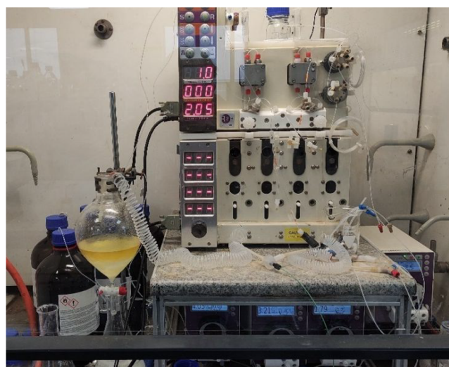
Figure 2. Flow apparatus designed for the continuous preparation of 2-benzoxazolinone ( 4 ).
