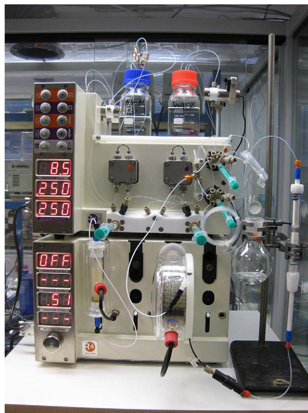
Figure 1. Vapourtec R2+R4 flow system.
