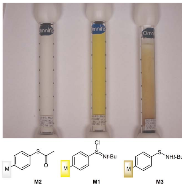
Figure 1 Thioacetate monolith M2 (left), N -( tert -butyl)phenylsulfonimidoyl chloride monolith M1 (centre), N -( tert -butyl)phenylsulfenamide monolith M3 (right)
