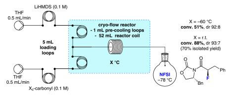
Scheme 3 Schematic of the flow apparatus for the preliminary assessment of a sequential addition quench protocol
