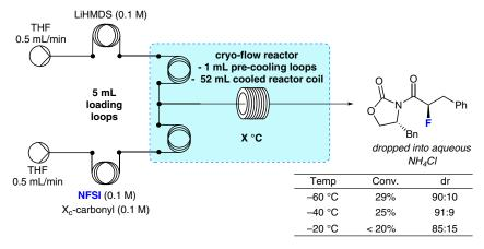
Scheme 2 Schematic of the flow apparatus for the in situ quench studies
