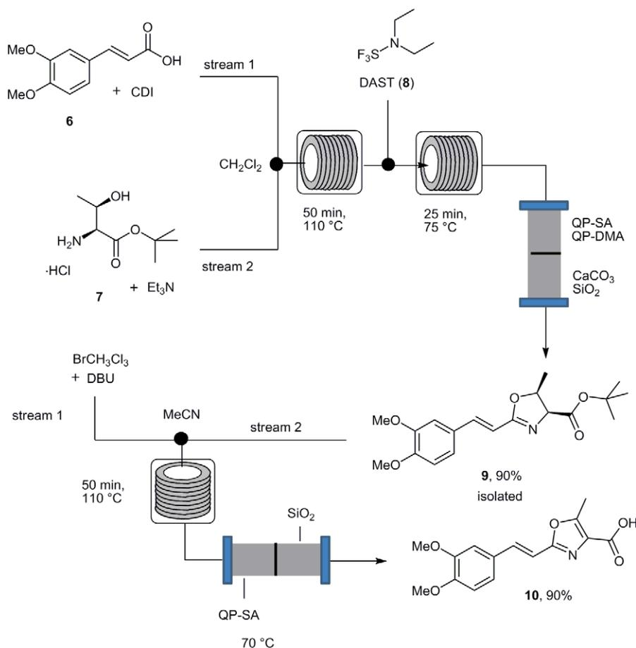
**Scheme 2** Flow synthesis of oxazole carboxylic acid **10**
