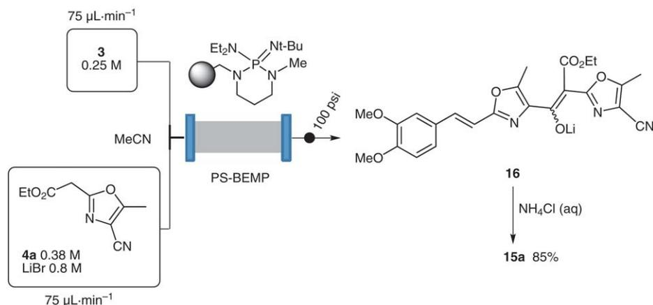
**Scheme 5** Claisen reaction of oxazole **3** and **4a** induced by PS-BEMP as polymer-supported base in the presence of LiBr
