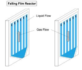
**Figure 3.** Falling film reactor with liquid flow falling downward and gas flowing either upward (left) or downward (right) above the liquid flow.
