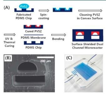
**Figure 7.** (A) Schematic illustration for the fabrication of a dual-channel microreactor with a poly(vinylsilazane) (PVSZ) shielded upper channel. (B) Cross-sectional view of dual microchannel with the PVSZ shielded upper channel. (C) The PVSZ shielded dual-channel microreactor filled with  $O_2$ , methylene blue (photosensitizer), and  $\alpha$ -terpinene (reagent). Reprinted with permission from ref 88. Copyright 2011 The Royal Society of Chemistry.
