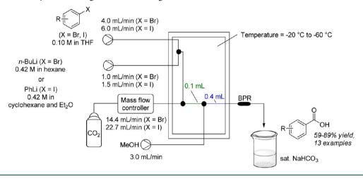
Scheme 20. Flow Setup for the Carboxylation of Lithiated Species Using CO<sub>2</sub> Gas
