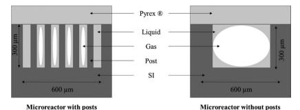
Figure 8. Cross-section of the microreactor showing a comparison of reactor with posts and reactor without posts under multiphase flow.
