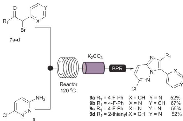
**Scheme 5** Flow synthesis of the imidazopyridazine cores.
