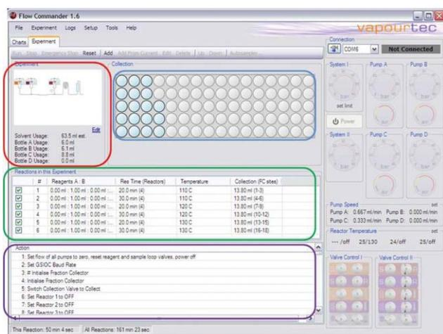
**Fig. 4** Screen shot of automatically populated optimisation table: system set-up, fraction collector rack, reaction conditions, action list.
