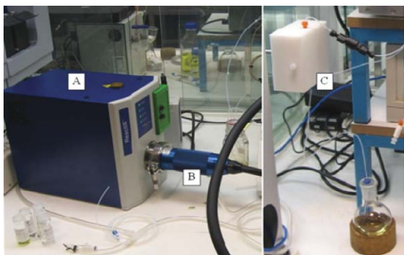
Fig. 2 A React IR 45 m. B Fibre optic cable. C Flow cell.
