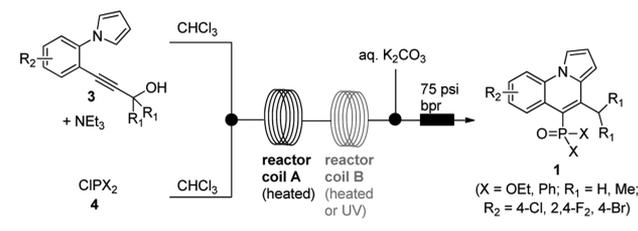
containing mixtures of the starting materials would combine in a T-piece prior to entering into a heated flow coil in which the cascade reaction would take place. Upon exiting the heated reactor the crude product stream would rapidly cool before being mixed with a quenching stream (aqueous K<sub>2</sub>CO<sub>3</sub>) and the product being collected (Scheme 6).
