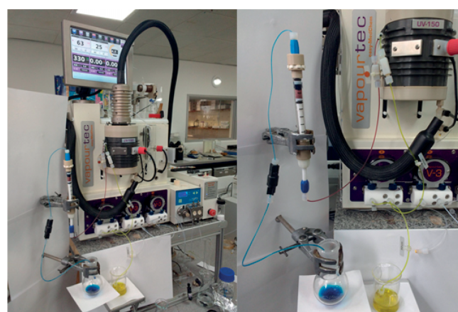
Figure 2. Photochemical colour change in the processing of phenazine salt 16 . (left to right) Starting material (SM), irradiated mixture 20 + 21 , product development upon basification in the presence of oxygen ( 6 + 1 ).
