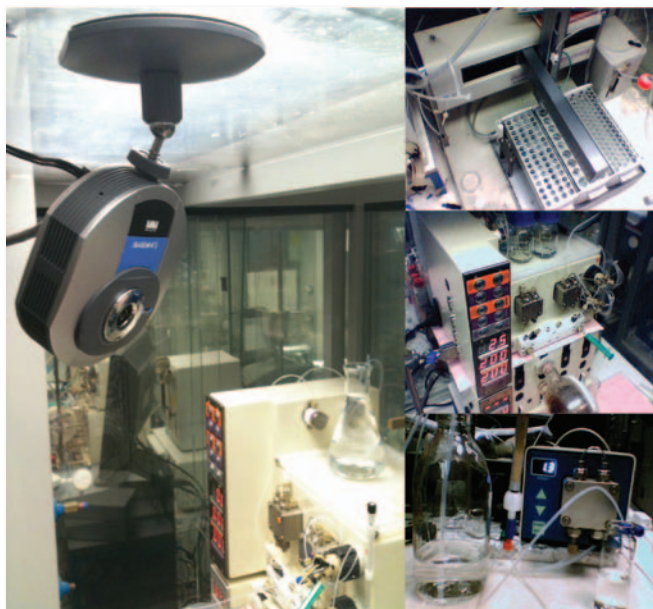
Figure 3. Webcam mounted in vented cabinet and live images captured during use.
