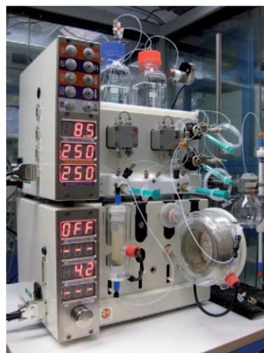
Figure 1. Vapourtec R2+/R4 flow system.
