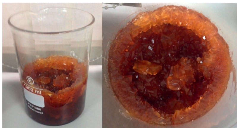
Figure 4. Crystallization of crude intermediate compound 2 upon standing at room temperature for two days.
