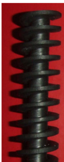
Fig. 5. Carbon impregnated PTFE (C/PTFE) microwave reactor insert.
